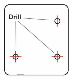
Figure 1: Mounting Plate Boring Template- Back View
