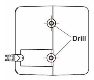
Figure 2: Mounting Plate Boring Template- Bottom View
